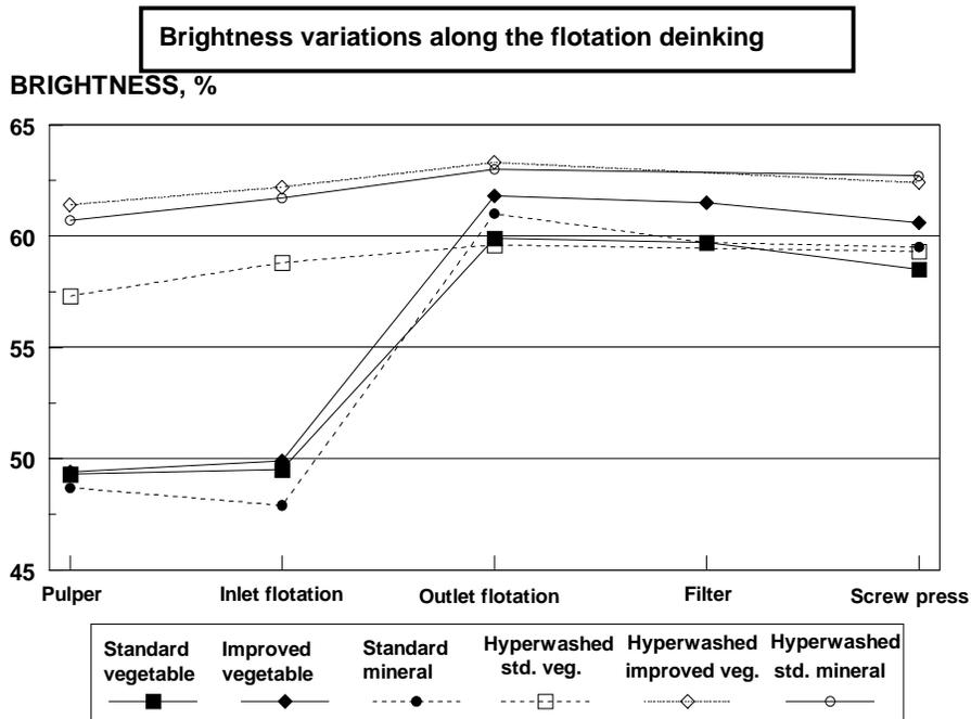
*Figure 2. Brightness variations along a conventional flotation deinking process for three newsprint inks on whole and hyperwashed pulps*
