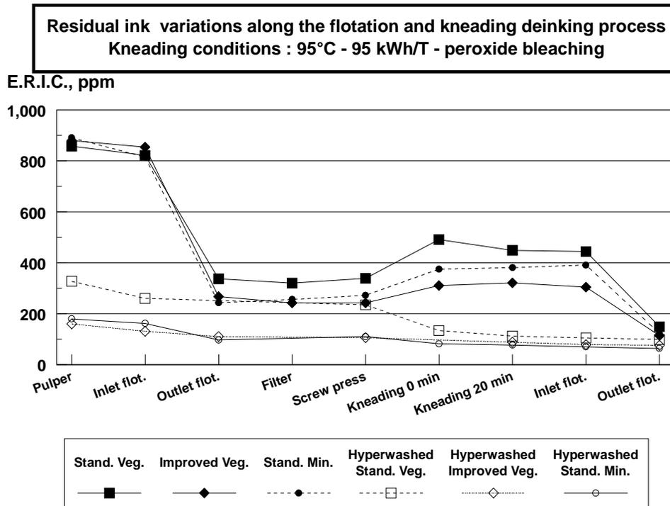
*Figure 5. Residual ink and ink detachment variations along a double-loop deinking process for three newsprint inks on whole and hyperwashed pulps (kneading conditions: 95 kW-h/metric ton at 95°C; peroxide bleaching)*
