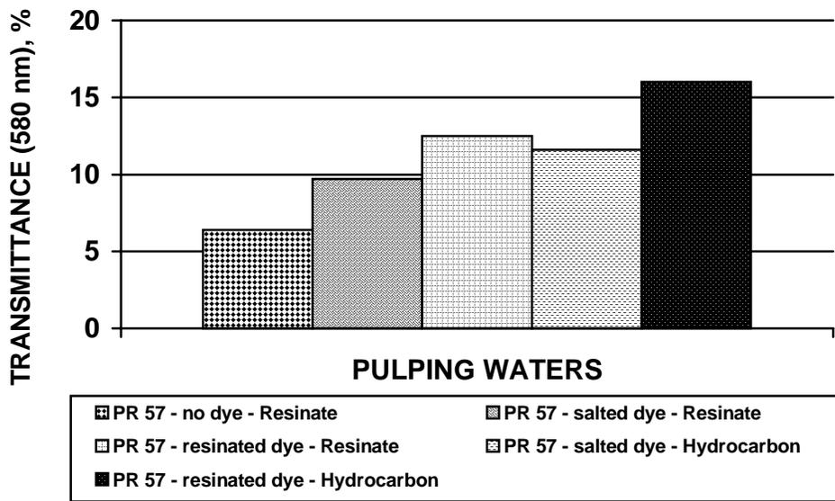
Figure 9. Influences of resin type and dye formulation on pulping water color for inks with dye
