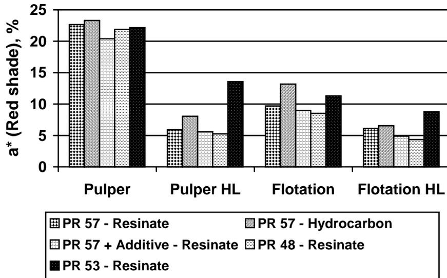
*Figure 6. Influences of resin type and pigment on pulp shade for inks without dye*
