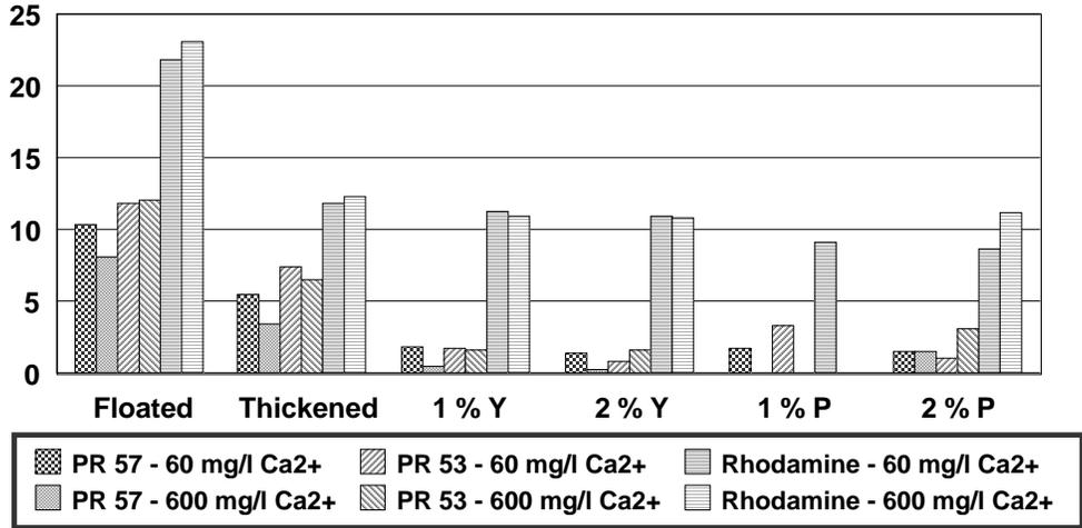
Figure 10. Color stripping: effects of peroxide (P) and hydrosulfite (Y) on pigments PR 57, PR 53, and rhodamine dye removal on entire pulp
