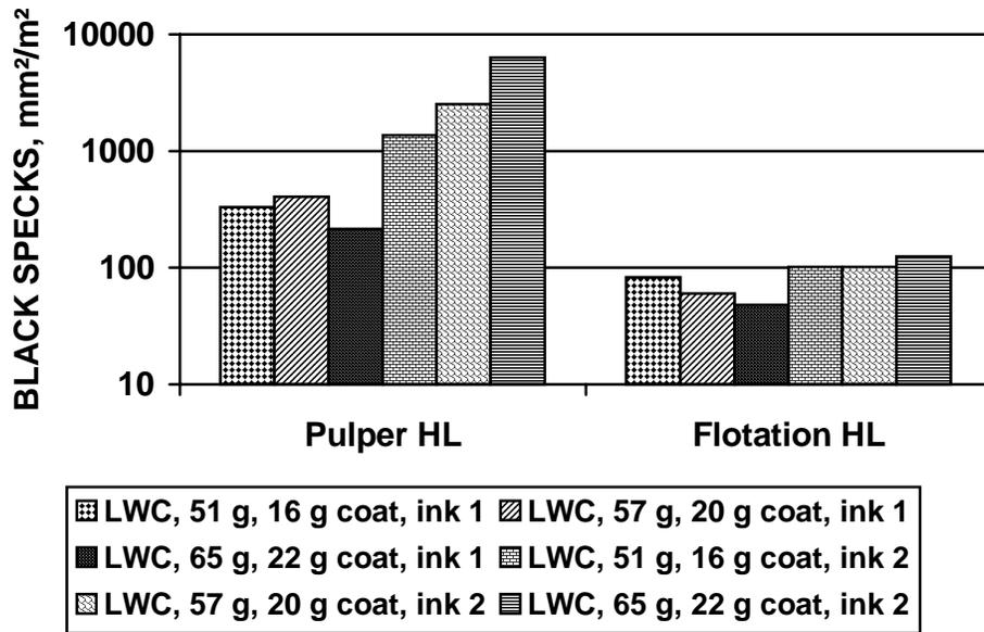
*Figure 14. Effect of different LWC paper on deinkability; speck contamination*
