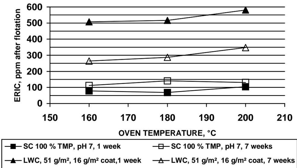
Figure 16. Effects of aging and drying temperature on residual ink after flotation
