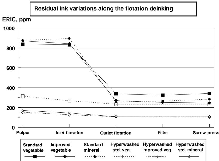
*Figure 3. Variation in effective residual ink concentration (ERIC) along a conventional deinking process for three newsprint inks on whole and hyperwashed pulps*
