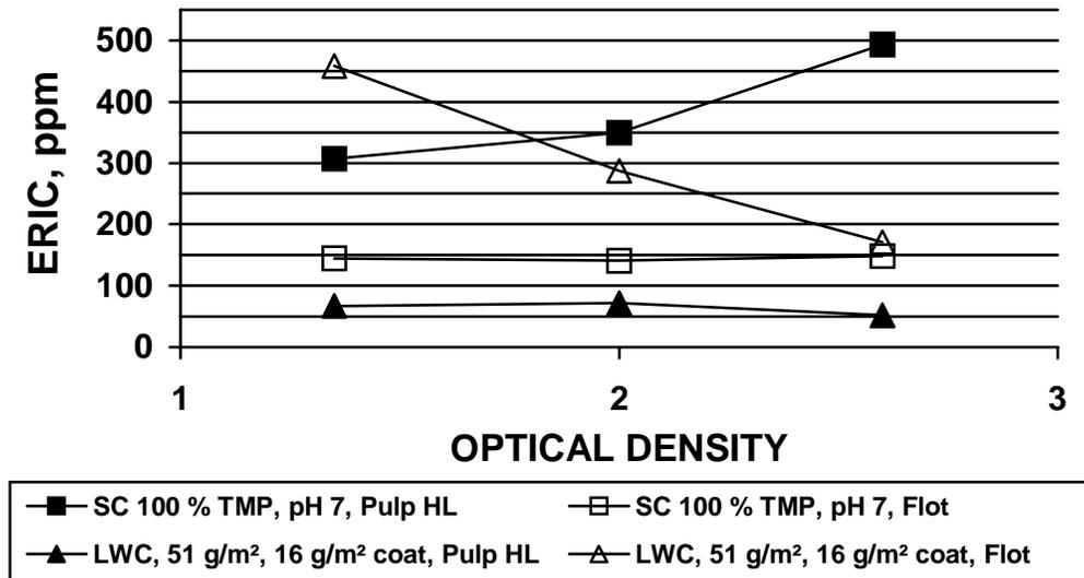
*Figure 19. Effects of base paper and ink thickness (through optical density) on residual attached ink (hyperwashed fibers) and on total ink content after flotation*
