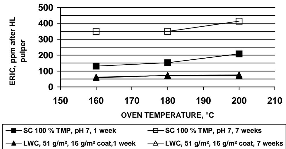
Figure 15. Effects of aging and drying temperature on residual attached ink on fibers
