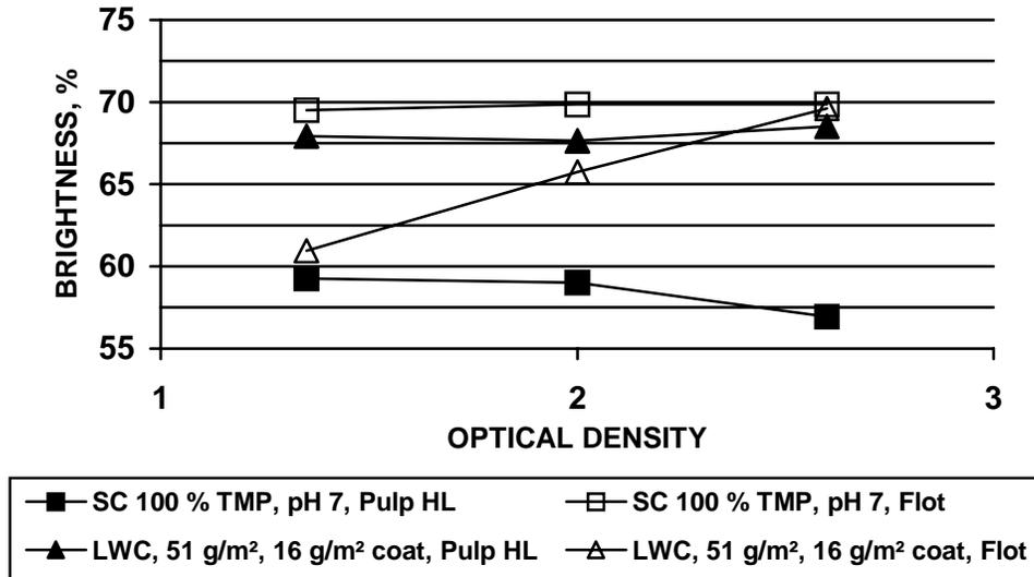
*Figure 18. Effects of base paper and ink thickness (through optical density) on brightness of hyperwashed fibers and on brightness after flotation*
