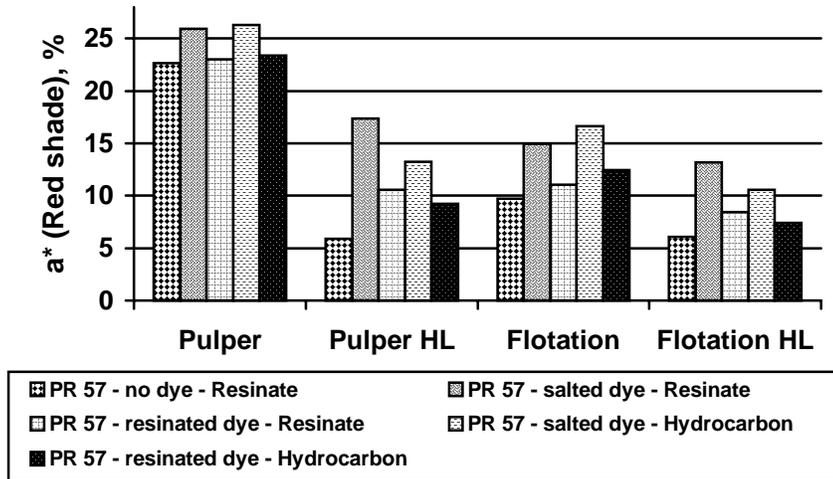
Figure 8. Influences of resin type and dye formulation on pulp shade for inks with dye
