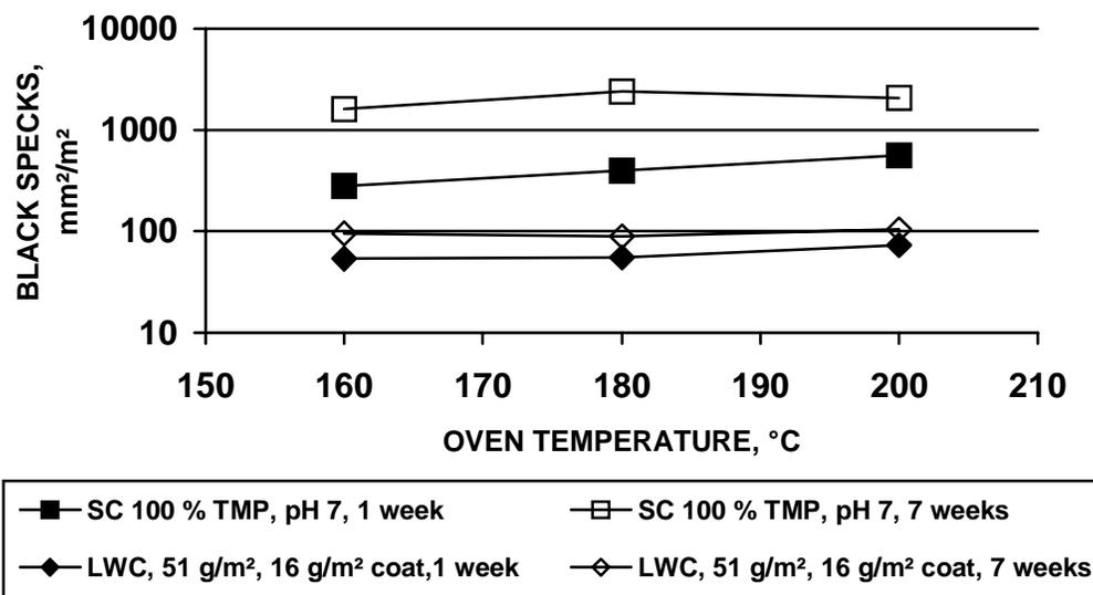
Figure 17. Effects of aging and drying temperature on speck contamination
