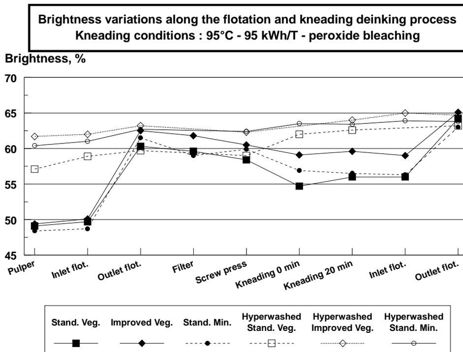
*Figure 4. Brightness variations along a double-loop deinking process for three newsprint inks on whole and hyperwashed pulps (kneading conditions: 95 kW-h/metric ton at 95°C; peroxide bleaching)*
