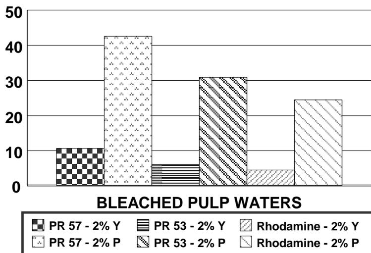
*Figure 12. Color stripping: effects of P and Y on pigments PR 57, PR 53, and rhodamine dye removal in bleached pulp waters*
