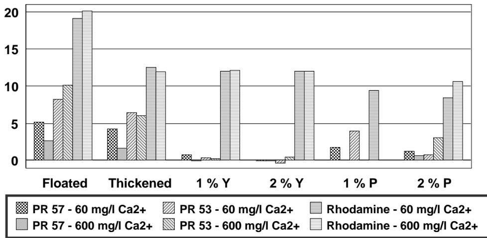
Figure 11. Color stripping: effects of P and Y on pigments PR 57, PR 53, and rhodamine dye removal on hyperwashed pulp
