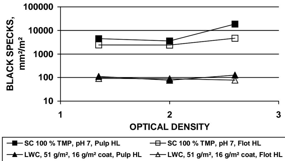
*Figure 20. Effects of base paper and ink thickness (through optical density) on speck contamination for hyperwashed pulp and after flotation*
