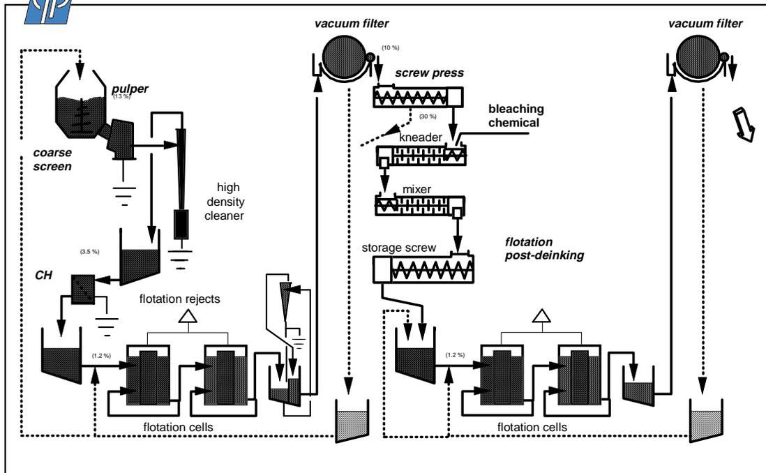
Figure A-1: Flow sheet of conventional flotation deinking process
